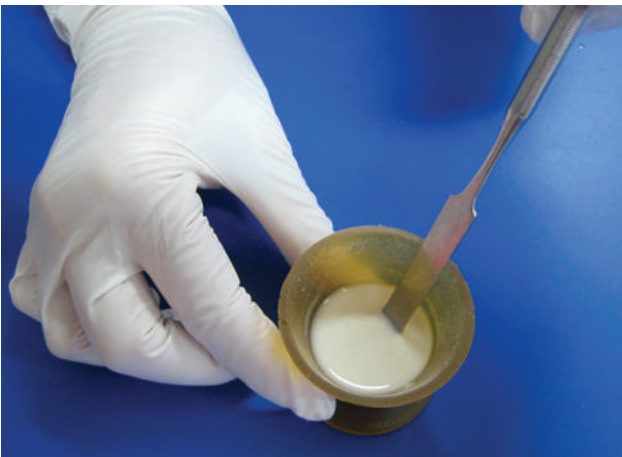
Figure 17. Mix the acrylic to manufacturer's specifications.
